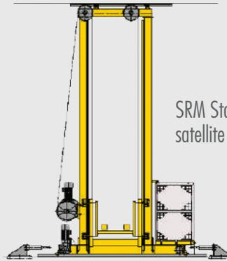
SRM Stacker crane with on-board satellite for multi-depth storage
