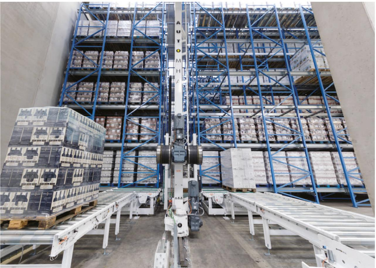
Stacker crane warehouses allow for the automated storage of loader units of all weights and sizes. The SRM stacker cranes are designed for solutions which make the most of available space while respecting the modes of handling requested.
