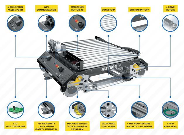
\*ADAPTABLE TOP, YOU CAN CHOOSE BETWEEN ROLLER CONVEYOR AND CHAIN CONVEYOR
