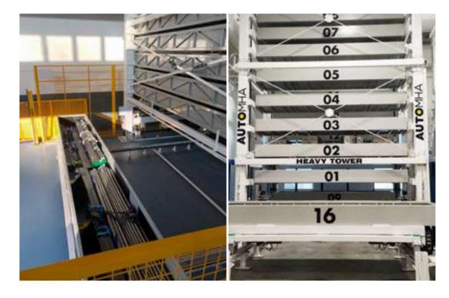
HeavyTower can be configured as an **inter-operational buffer** and used alongside cutting and production machines. Automha's **HeavyTower** is the ideal solution for storing steel bars and profiles, tubes, heavy accessories, semi-processed items, parts, molds and large items in general.
