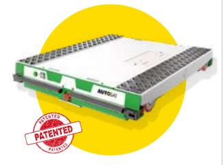
Autosat is equipped with a special removeable lithium battery weighing 9 kg with a discharge time of up to 10 hours, and is controlled by multifunctional radio control.
